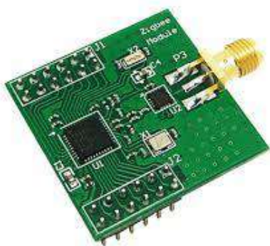
Fig. 6. Module base on chip CC2530
