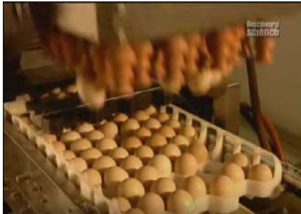
Fig. 4. Fragment of installation of Inovoject (automatic removal of eggs with dead embryos).
