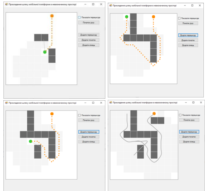
Fig. 3. Example of the algorithm in the first steps and the result of paving the way.
