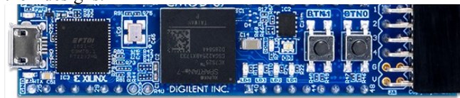
Fig. 1. Xilinx Educational FPGA Board: Cmod S7 FPGA
