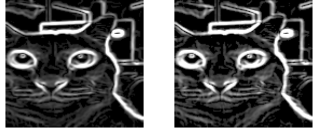
Fig. 3. Sobel edge map of a 128×128 test image: the scalar baseline (left) and the optimized Helium implementation (right) are visually similar, despite the large nominal max-error caused by threshold flips.
